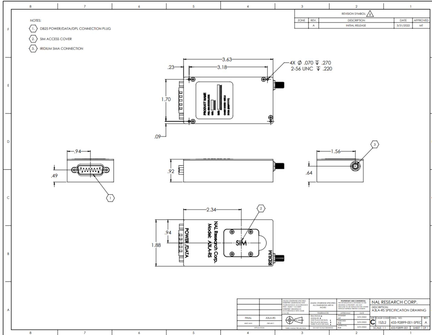
Figure 12: AL3A-RS Mechanical Drawing
