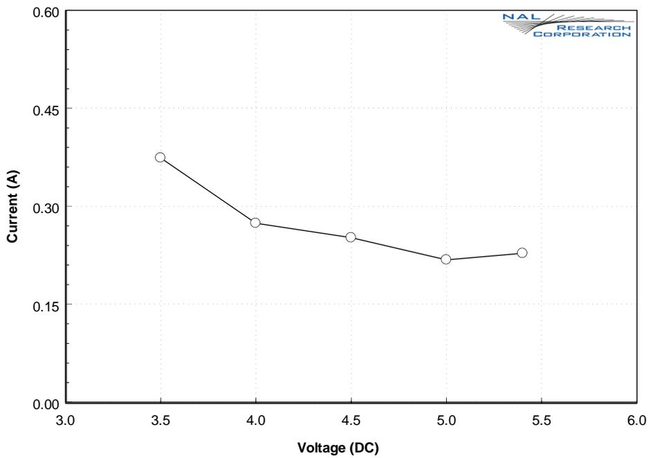
**Figure 5: Average Current Drawn During an SMS Transmission**
